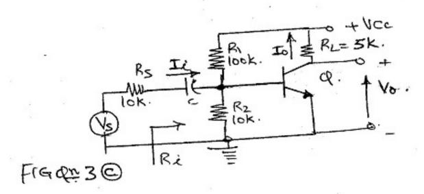
**4.** (a) i) Draw the hybrid  $-\pi$ , circuit at low frequencies, if the load resistance is  $R_L=\frac{1}{g_L}$ , Prove that
